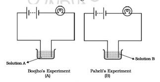
They found that the bulb in the setup A glows more brightly as compared to that of the setup B. You would conclude that
