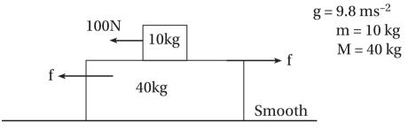
$f = \mu mg = 0.4 \times 10 \times 9.8 = 39.2 \text{ N}$  acceleration of 40 kg block
