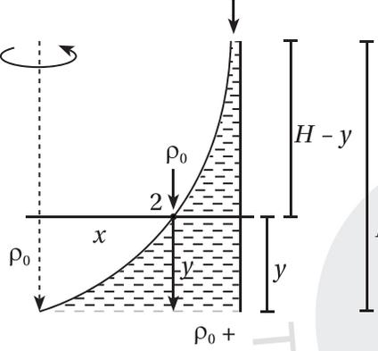
$\rho_0 = \rho_0 + \rho g y - \frac{1}{2} \rho (\omega x)^2$ $\therefore y = \frac{\omega^2 x^2}{2g}$ <p>If the fluid is rotating, write <math>+\left(\frac{1}{2}\rho\omega^2 x^2\right)</math> while moving away from the axis and <math>\left(-\frac{\rho\omega^2 x^2}{2}\right)</math> in moving towards the axis.</p> <p><math>y = 2 \text{ cm}</math></p> |  |
