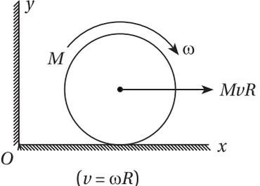
$L_0 = MvR + I\omega = MvR + \frac{1}{2}MR^2\omega = \left(\frac{3}{2}\right)MR^2\omega$                                        |  |
